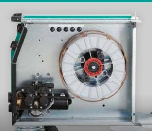
The wire feed system and wire spool mounting points are both open and easy to access.
